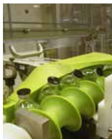
Conveyor screws made of TECAGLIDE enable a shock free and silent process.
